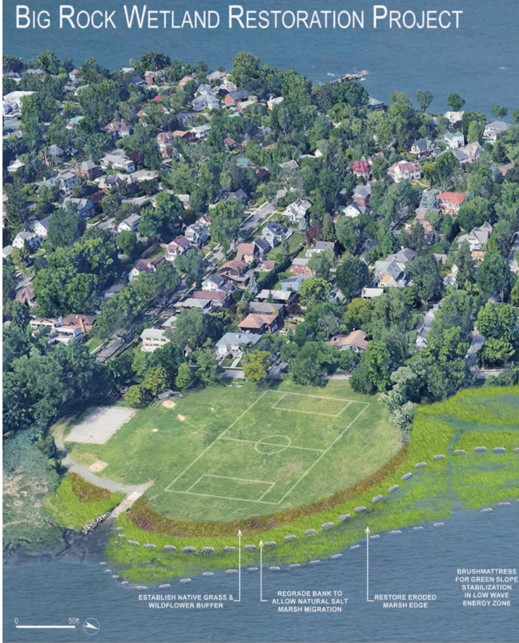
An aerial view rendering of the $2.1 million Big Rock Restoration Project showing the entire 7 acre site
